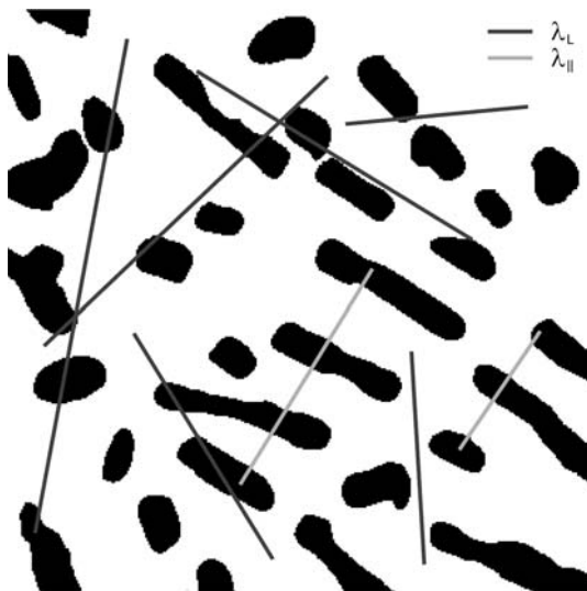
Fig. 2 Schematic demonstrating the calculation of the parallel and random line spacing measurements. The \lambda_{||} measurement is determined by drawing lines perpendicular to parallel silicon plates while the \lambda_L measurement involves the generation of random lines over the eutectic area
